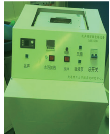
图4 兆声电铸设备 Fig.4 Megasonic electroforming equipment
